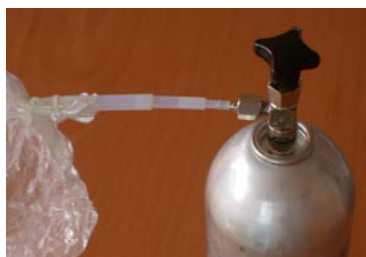
picture 6: Sampling bag connected to gas can
